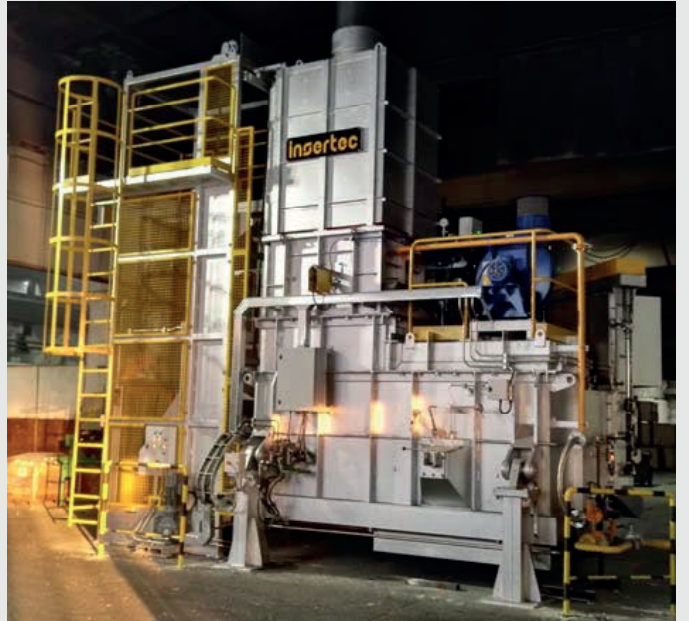
General view Tilting MELTOWER 1000 kg/hr
