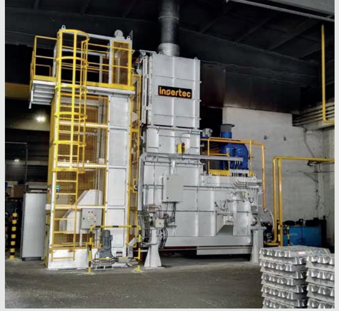
General view Tilting MELTOWER 1000 kg/hr
