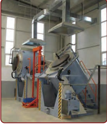
Gas or Electrical Heated Hydraulic Tilted Aluminium Melting Furnaces
